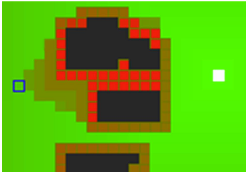
Fig. 2.5. Illustration of an artificial potential field for obstacle avoidance
