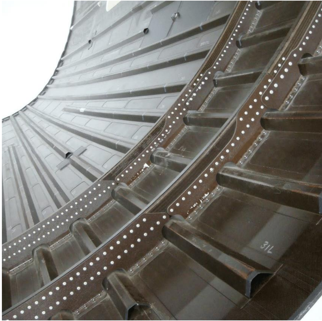
Fig. 2.3. The panel of the composite airplane Boeing 787
