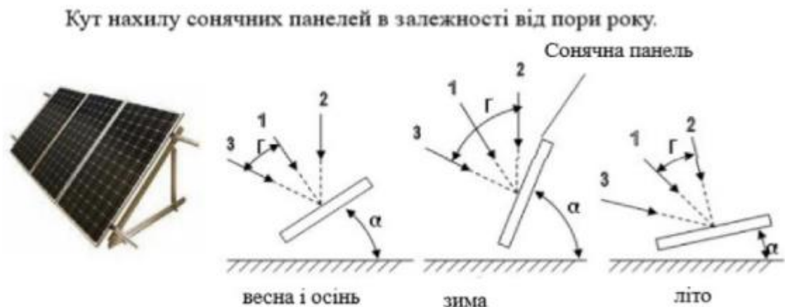
Fig.1.7. Recommendations for the angle of inclination of solar panels, depending on the season
