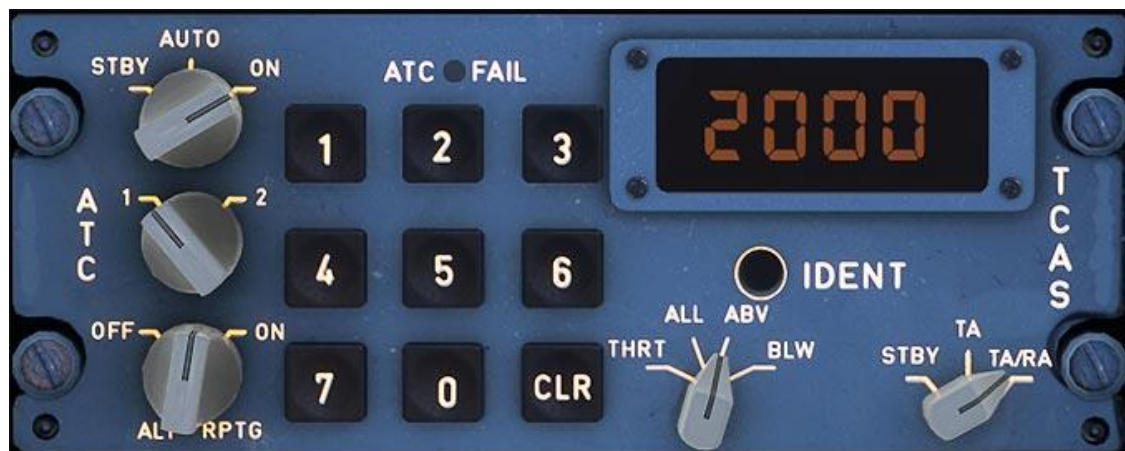
Fig. 1.3 ATC/TCAS control panel of Airbus A320 airliner, showing the TCAS mode control knob (bottom-right).
