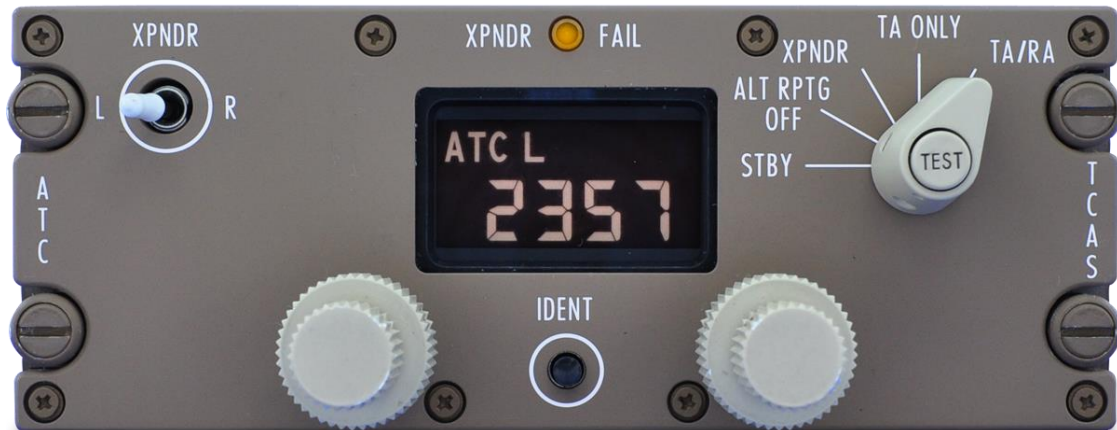
Fig. 1.2 ATC/TCAS control panel of Boeing B737 airliner, showing the TCAS mode control knob (top-right).
