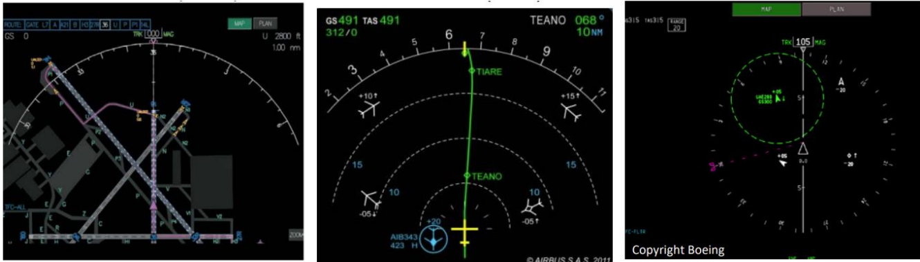
Fig. 1.7 Applications of ADS-B; SURF (left), AIRB (middle), and VSA (right).
